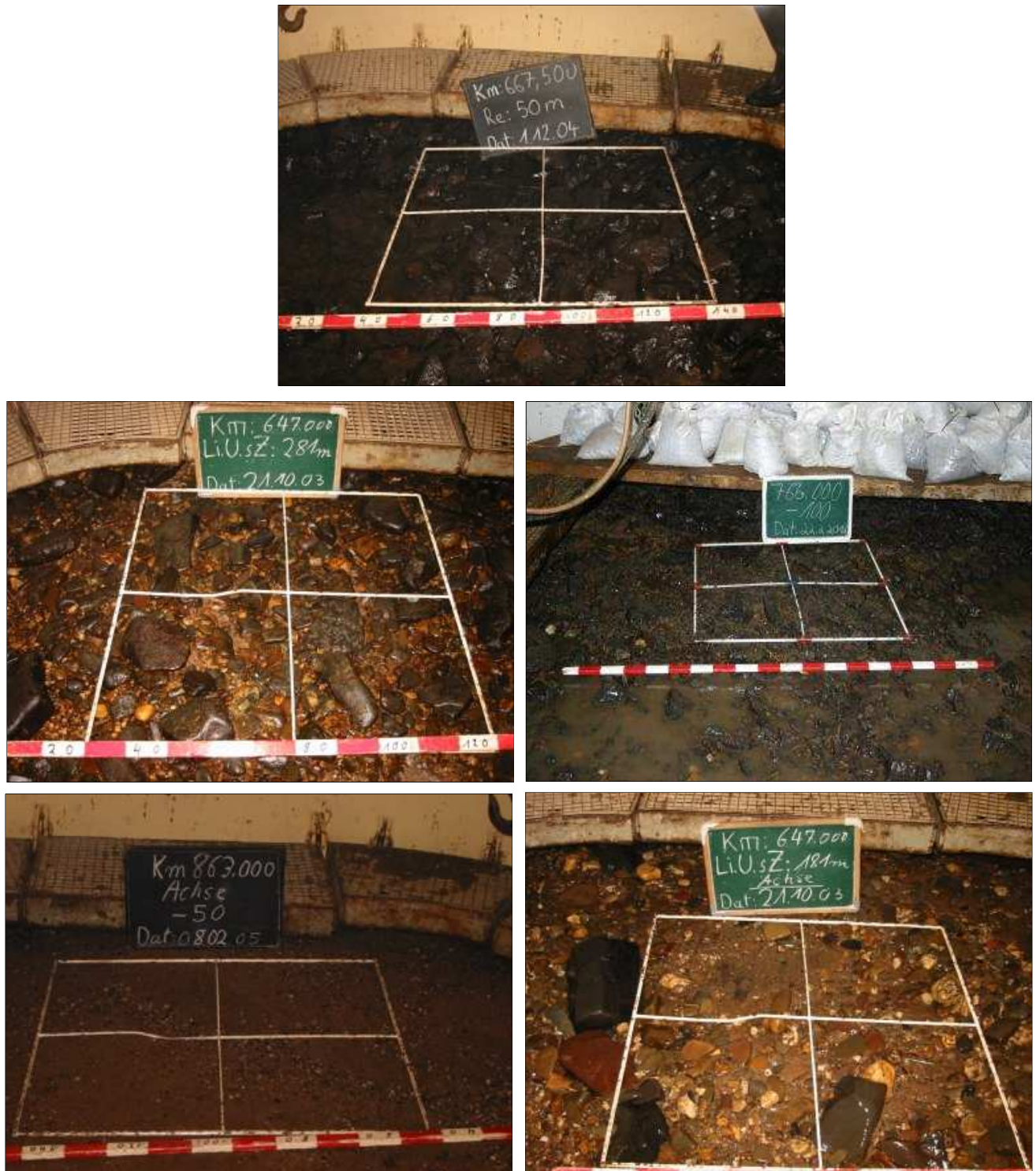
Figure 4.4.2 Exemplary in situ-photographs of substrate samples on the Rhine's river bed which were used for granulometric analysis (compare table 4.4.1)
